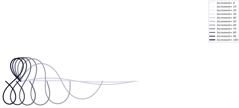
Figure 44: Column buckling mode 2: animation frames for different increments
