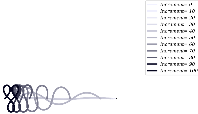
Figure 47: Column buckling mode 3: animation frames for different increments
